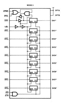
Figure 6. Talker/Listener/Controller Data Configuration
